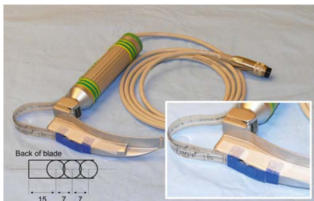
Fig. 1. Macintosh laryngoscope with sensors attached; detail of the placement of the Flexiforce (Tekscan, Boston, MA, USA) sensors used. The schematic shows the location of the sensors toward the rear of the laryngoscope blade
